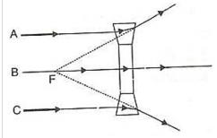
As shown in the figure the concave lens has two glass prisms and one glass block. One of the glass prisms is situated above the glass block and one below the block.
