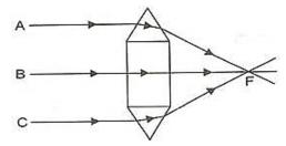
As shown in the figure the convex lens has two glass prisms and one glass block. One of the glass prisms is situated above the glass block and one below the block.
