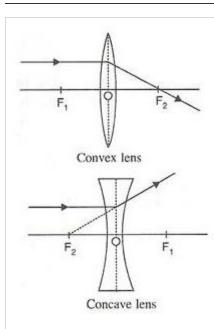
(iii) A ray of light passing through the first focus  $F_1$  (in a convex lens) or directed towards the first focus  $F_1$  (in a concave lens), emerges parallel to the principal axis after refraction.
