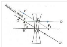
(ii) When object (AB) is situated at any point between infinity and optical centre of the lens then image forms between focus and optical centre. This image is diminished in size and virtual and upright.
