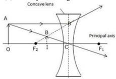
(c)The focal length is measured from optical centre C to F<sub>2</sub>.
