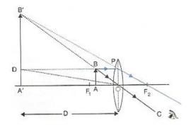
The image formed will be virtual, magnified and erect.
