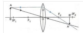
Here the candle is AB and its real and inverted image is formed between F<sub>2</sub> and 2F<sub>2</sub>.
